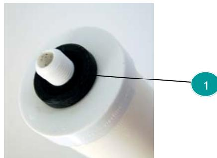
6. Check the new cartridge and the sealing washer (1) is correctly positioned. Check that the 'O' Seal inset in the top of the head (2) is correctly positioned. Screw the cartridge into the head until you feel the resistance of the washer meeting the sealing face. Continue to screw the cartridge a further  $\frac{1}{4}$  turn to make an effective seal. **Important note.** Do not be tempted to over tighten the cartridge; over tightening will distort the sealing ring.
