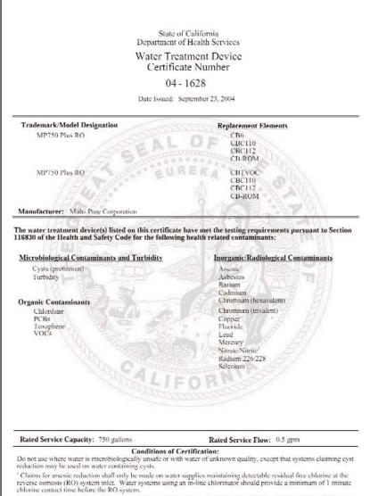
This system is acceptable for treatment of influent concentrations of no more than 27 mg/L nitrate and 3 mg/L nitrite in combination measured as N and is certified for nitrate intrite reduction only for water supplies with a pressure of 280 kPa (40 psig) or greater. A sampling and analysis test kit for nitrate is provided for checking the performance of this system. Frequent analysis is encouraged.
