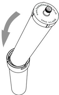
5. Holding the sump over the sink remove the spent cartridge and empty the water in the sump. Dispose of the spent cartridge. Place the new cartridge in the sump.
