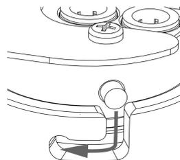
6. Refit the sump to the housing head by engaging the pins in the slots and turning the sump to the right until it is fully engaged.
