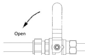
7. Turn on the water supply and check the system carefully for leaks. Leave the tap in the 'on' position and allow the water to run for a minimum of 10 minutes to flush the filter. Check the flow rate. We recommend no more than 30 seconds a litre for optimum performance. If the flow is too fast it can be regulated by adjusting the stop valve.
