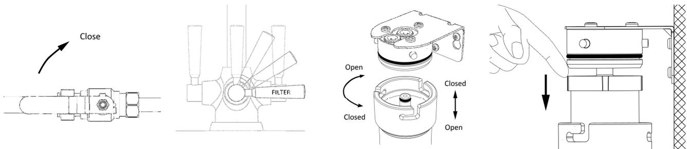
1. Locate the shut-off valve and turn off the mains water supply to the filter housing.
